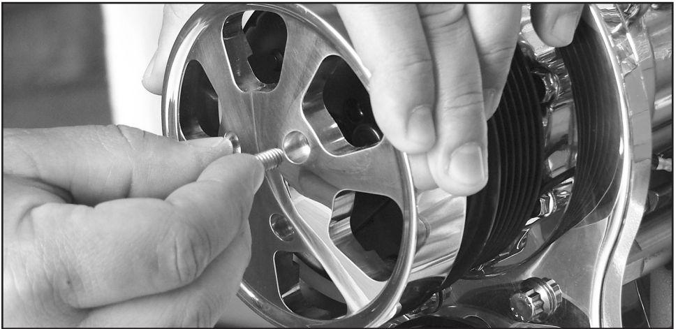
Figure 13: Install SD-7 Compressor Clutch Cover
