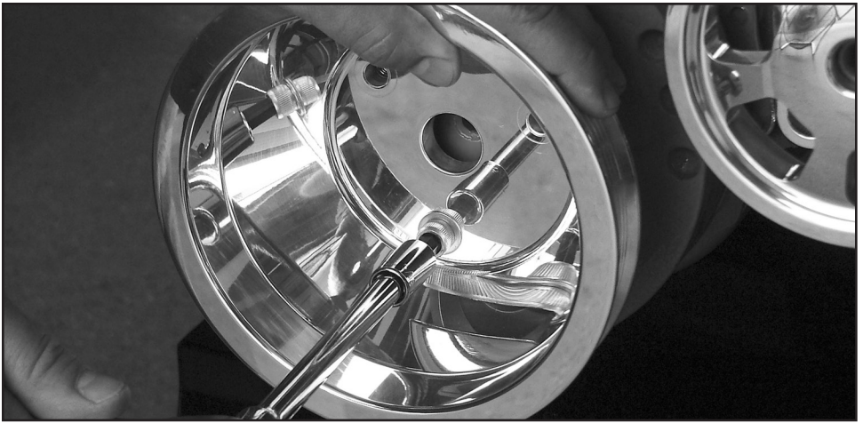
Figure 12: Install Crankshaft Pulley
