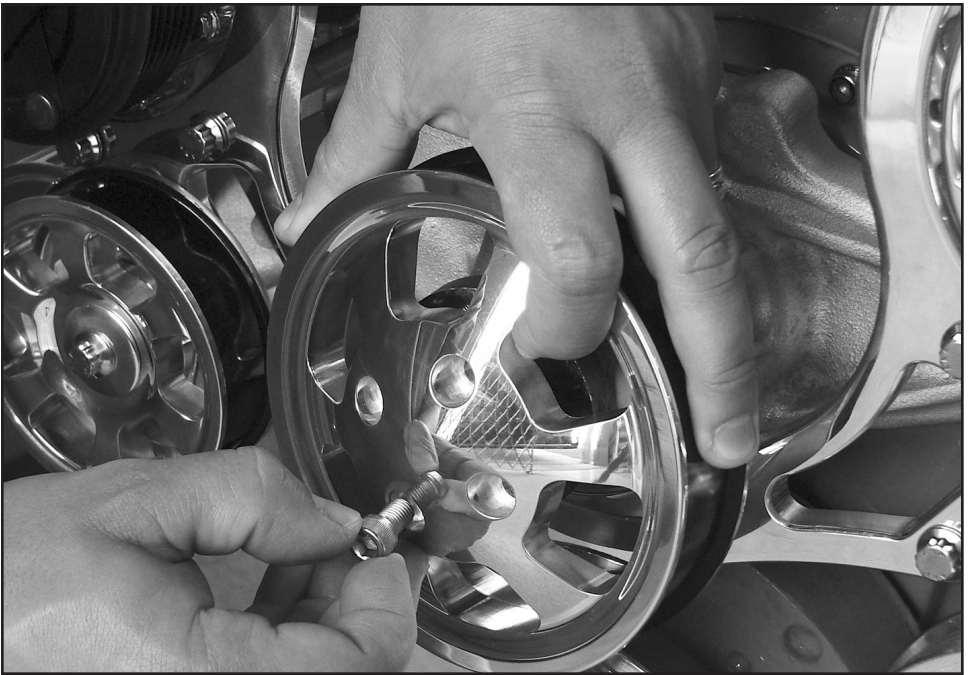
Figure 11: Install Water Pump Pulley onto Pump
